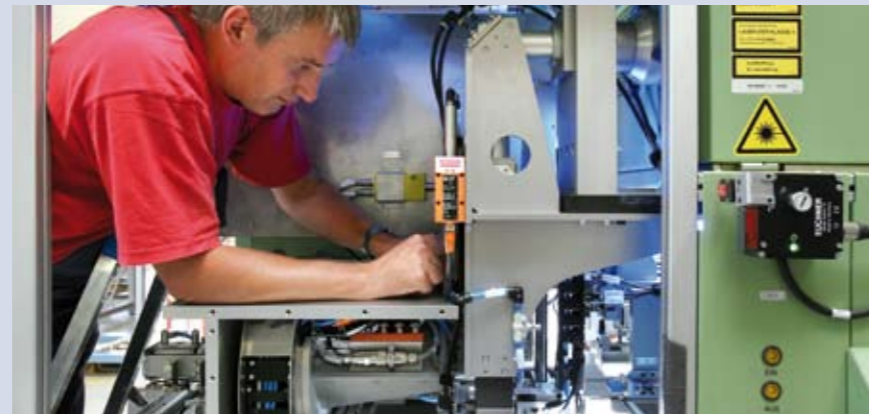
Installation of a laser welding unit as a part of a complex assembly line
