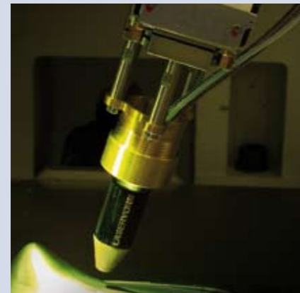
Fully automated laser cladding process with concentric powder injector
