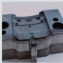
Repair of die casting molds by using laser cladding treatment
