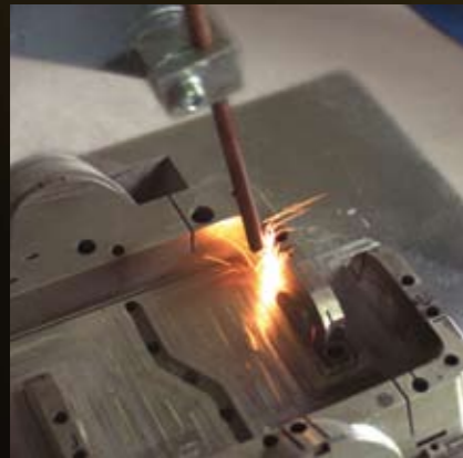
Laser cladding with powder for modification of an injection molding
