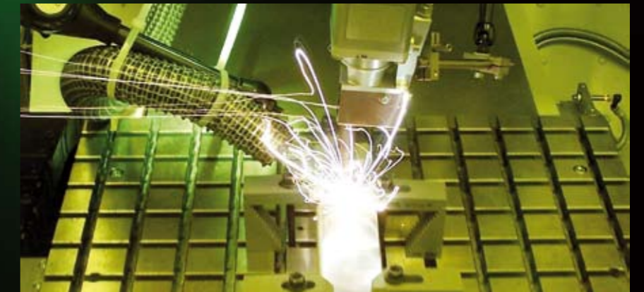
Laser welding of aluminum with fiber laser
