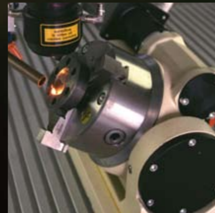
Pyrometer adjusted laser hardening
