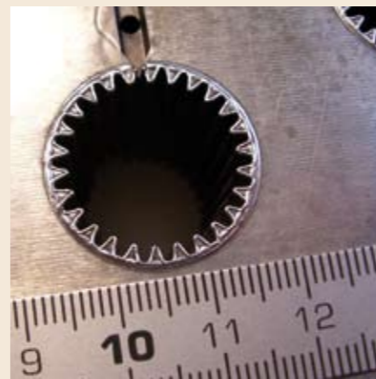
Precision laser cladding on die casting molds
