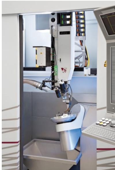
Fig. 2 LV Midi with five axes and LV SpinScan for real 3D treatment.
