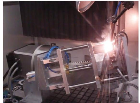
Fig. 1 Programmable beam quality bridges gaps while welding exhaust parts.
