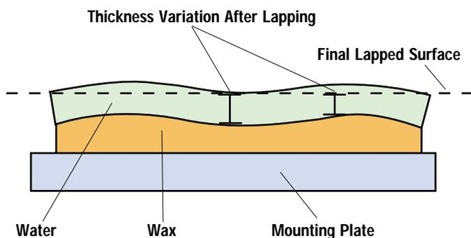
Figure 1. Effect of an uneven wax layer.
