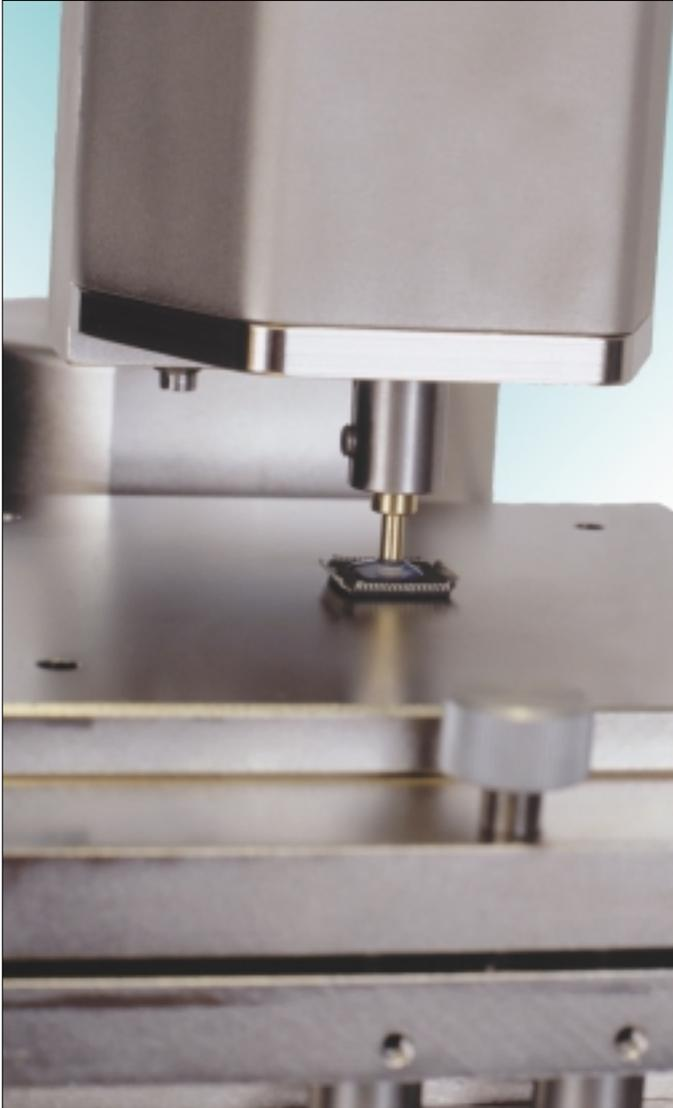
Backside selected area polishing of an electronic package. This technique can be used to thin ceramic and plastic packages, as well as unencapsulated semiconductor wafers.
