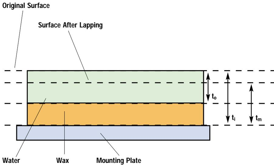
**Figure 2.** Thickness measurement.
