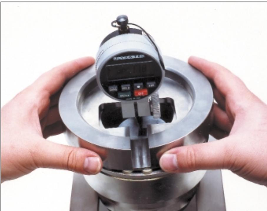
A precision micromount allows for initial set-up and alignment of the wafer. It also allows for accurate measurement of the amount of material removed during back lapping.
